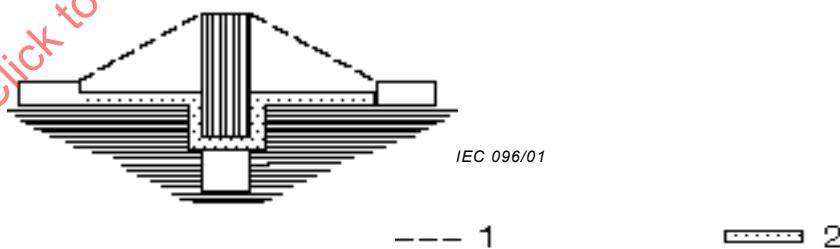
Condition: Creepage distance through uncemented joint is less than creepage distance over barrier
