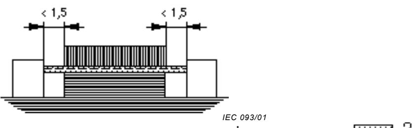
Condition: Path under consideration includes an uncemented joint with grooves less than 1,5 mm wide on each side
