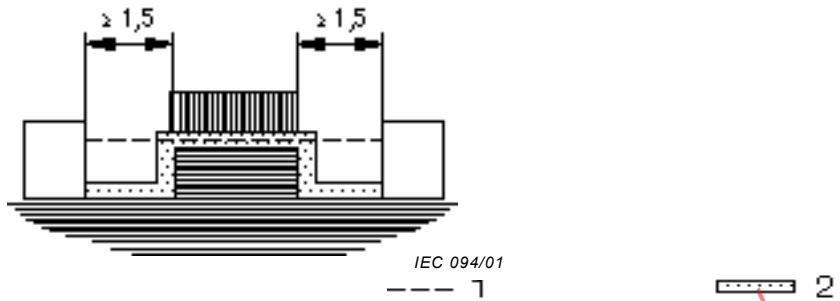
Condition: Path under consideration includes an uncemented joint with grooves equal to or more than 1,5 mm wide on each side
