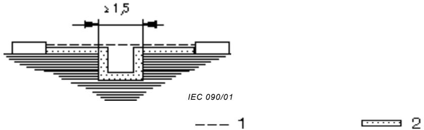
Condition: Path under consideration includes a parallel-sided groove of any depth  $d$  equal to or more than 1,5 mm
