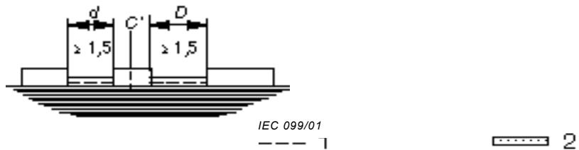
C—conductive part interposed in the insulating path between the conductors.
