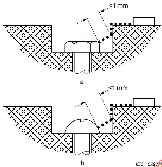
Gap between head of screw and wall of recess too narrow to be taken into account.
