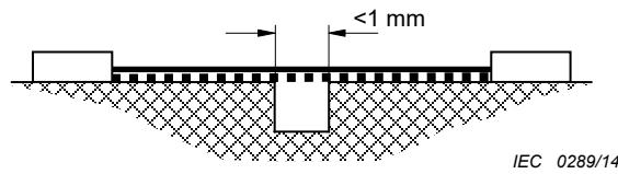
Condition: Path under consideration includes a parallel or converging sided groove of any depth with a width less than 1 mm.
