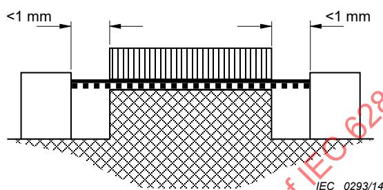
Condition: Path under consideration includes an un cemented joint with grooves less than 1 mm wide on either side (0,25 mm for dirt-free situations).
