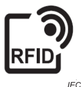
Figure 5 – Marking of a RFID transponder as a digital nameplate
