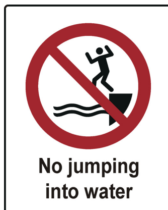
Figure D.1 — Water safety sign (ISO 20712-1-WSP014) with supplementary text
