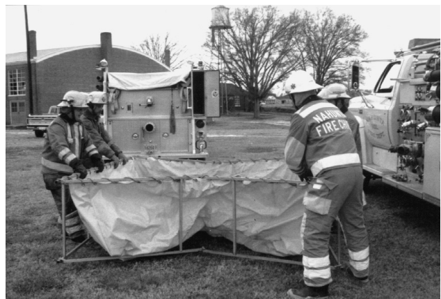
FIGURE C.1.13(a) Fire fighters setting up portable drop tank. (Courtesy of Nahunta Volunteer Fire Department, NC)
