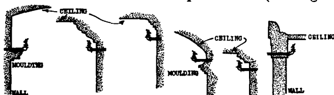
Fig. 4450. Suggested Arrangements for Sidewall Sprinklers — placed to receive early heat waves and provide effective distribution.
