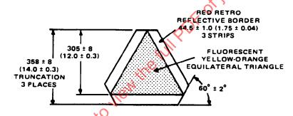
DIMENSIONS ARE IN MILLIMETERS WITH INCH EQUIVALENTS IN PARENTHESES.
