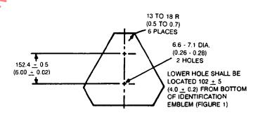
DIMENSIONS ARE IN MILLIMETERS WITH INCH EQUIVALENTS IN PARENTHESES. BACKING MATERIAL SHALL BE AS LARGE AS OR LARGER THAN THE IDENTIFICATION EMBLEM (FIGURE 1)
