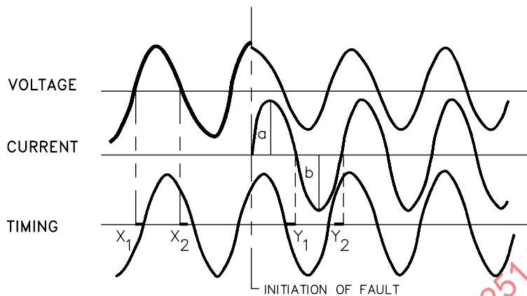
$$\text{Current} = \frac{a+b}{2} \text{ rms calibration of instrument element}$$
